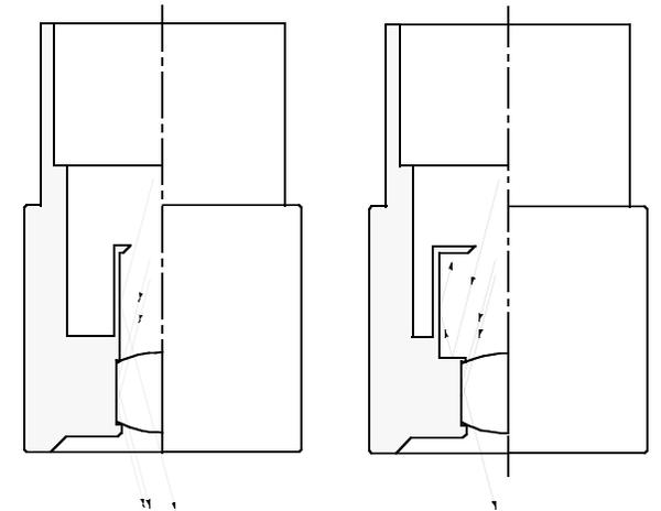
Changing geometry of internal parts and blackening lens edges may dramatically reduce unneeded reflections.
