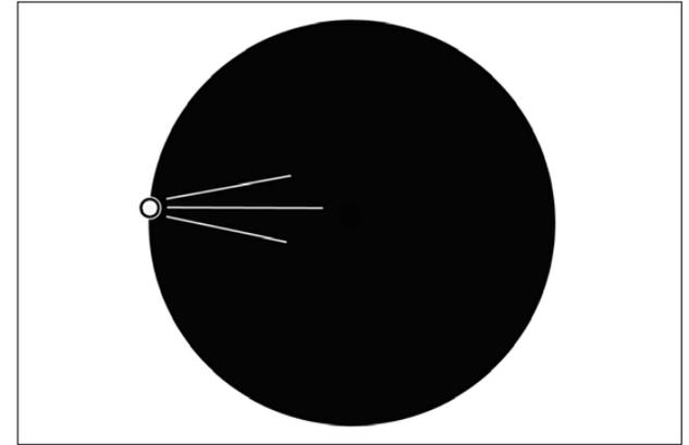
To check internal reflections, scatter, ghosting, etc. the light source was setup for higher brightness. Most unnecessary reflections appears in the FOV at the moment as a splash of light or ghost when the Airy disc is going behind the edge of FOV.
