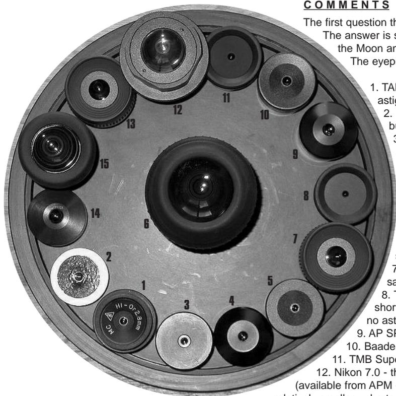
1. TAK Hi-Ortho 2.8 - highest power eyepiece tested, no defocusing on the edge, but very small astigmatism.
