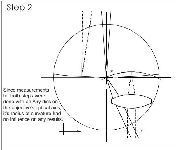
For the second measurement the eyepiece was shifted to the position when the Airy disc was near the edge of FOV and focused on the Airy disc image (if required).
