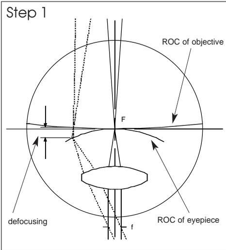
The first measurement was done with an eyepiece position on the axis - Airy discs at the center of FOV.
